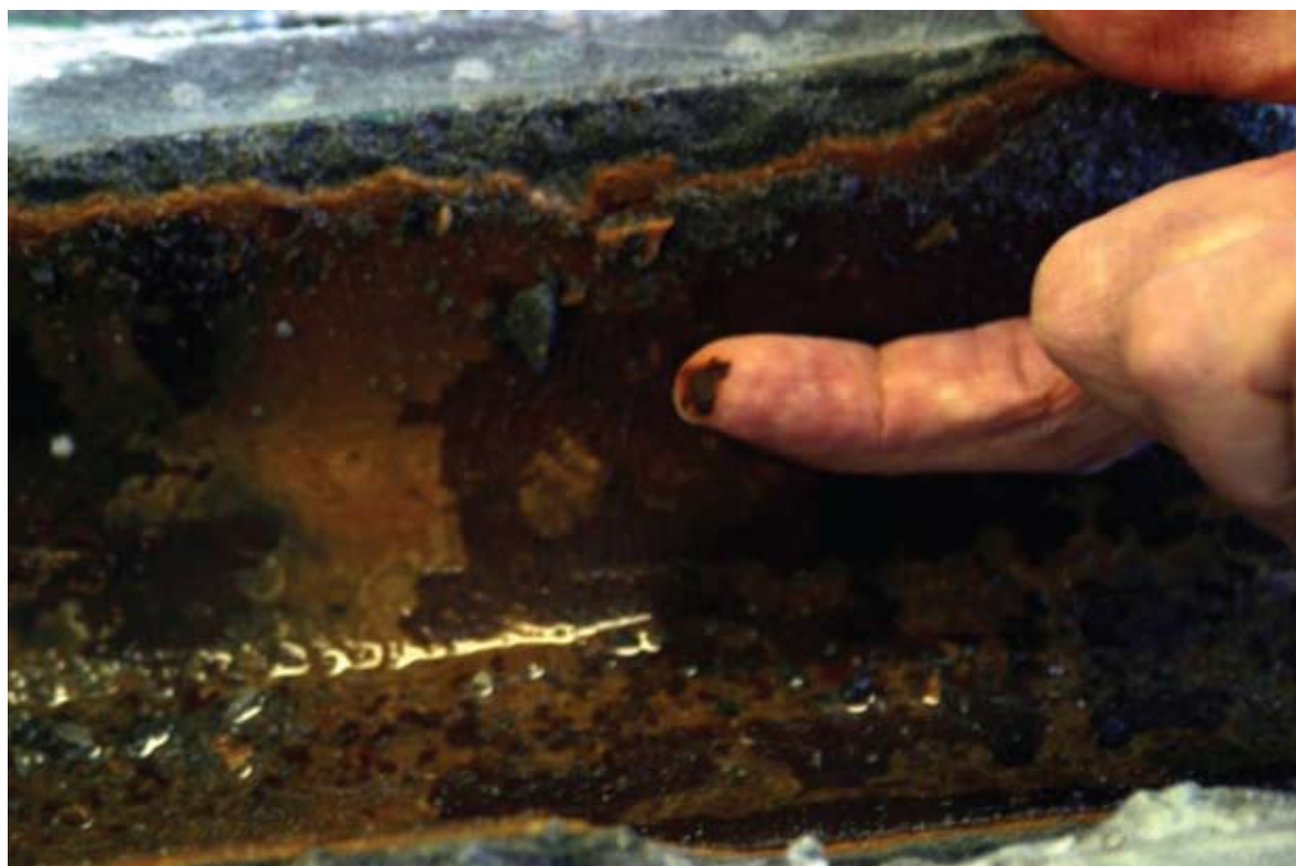
Figure 3. Photograph of a mature biofilm with metal-rich upper layer above a biomass-rich lower layer on the pipewall surface within a distribution system (photo by Luke Zappia).
